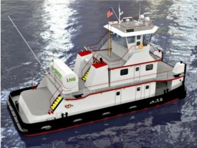
Concept rendering of towboat following conversion to burn LNG as a marine fuel The Shearer Group Inc
